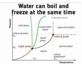
It is called the 'triple point', and it occurs when the temperature and pressure is just right for the three phases (gas, liquid, and solid) of a substance to coexist in thermodynamic equilibrium.
