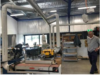
This pipework will deliver all the dust to two filter bags which can be seen at the rear, looking like condoms.
