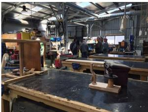
The Peninsula North Men's Shed is well equipped and has a large kitchen/ meeting room. They have a dust extraction system which they installed themselves at a cost of \$10,000, \$8000 for the extractor and \$2000 for pipework and fittings. They also have a reticulated compressed air system. Thanks to John Thornton for driving us.
